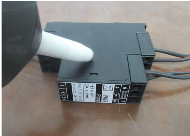
Picture 3.1. A – Air discharge
